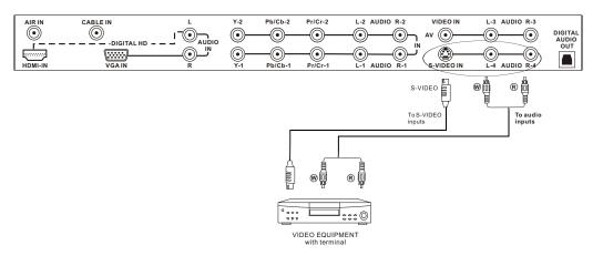
1.Turn off the power to the LCD TV and VCR or video camera.
